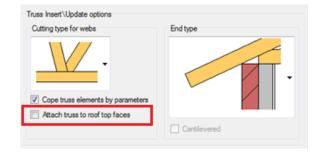
• Cut/Cope truss elements by selected cut type.
