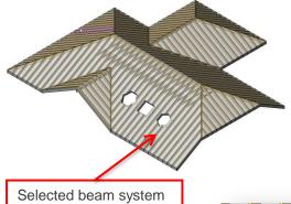
Selected beam system with three openings.
