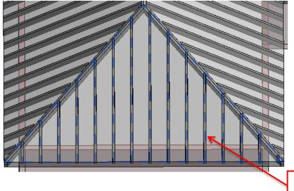
As you can see, the common rafter beam system is recreated. The cuts in connections and ends are not updated and there is no opening. For this slope, you have to run the required functions again.
