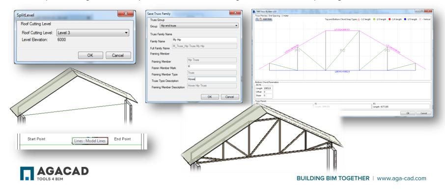
Truss Builder works well in case of multi pitched roofs too.
