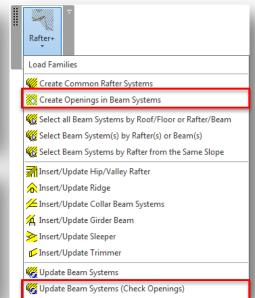
If opening position changes, just repeat the function Create Openings lin Beam Systems and beam systems will be updated according to new openings positions.
